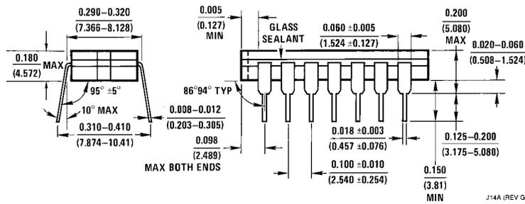
**14-Lead Ceramic Dual-In-Line Package (J)**
