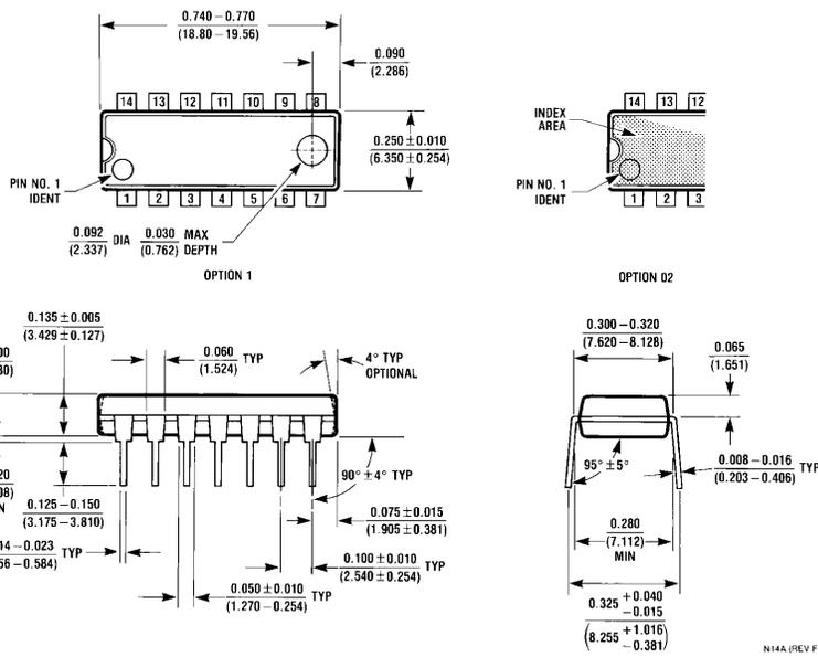
**14-Lead Molded Dual-In-Line Package (N)**
