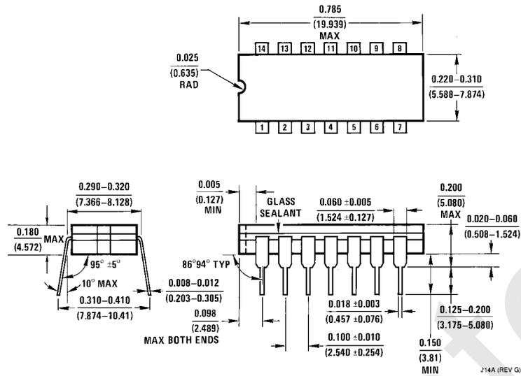
**14-Lead Ceramic Dual-In-Line Package (J)**
