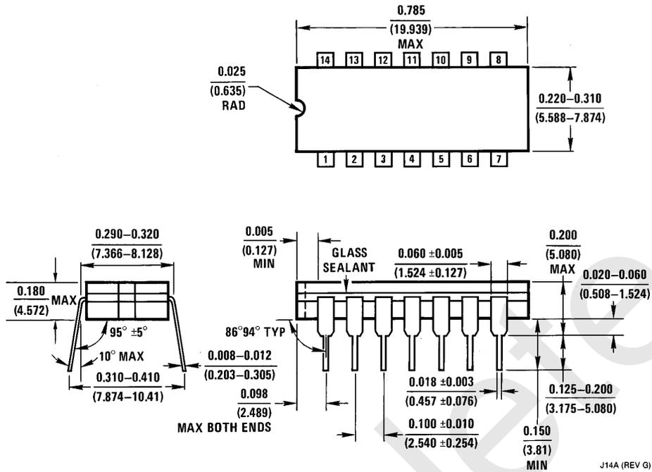
14-Lead Ceramic Dual-In-Line Package (J)
