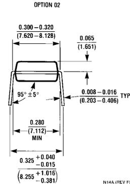
**14-Lead Molded Dual-In-Line Package (N)**
