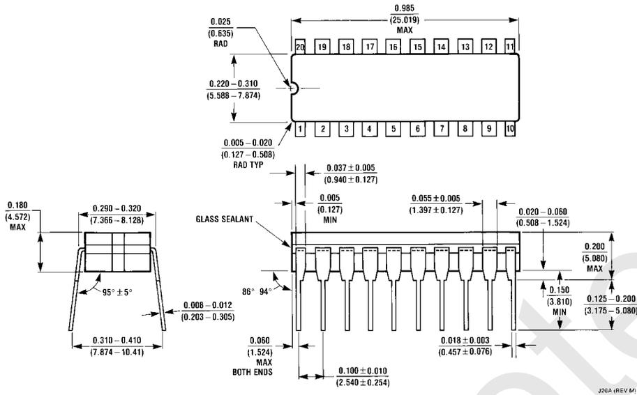
**20-Lead Ceramic Dual-In-Line Package (J)**
