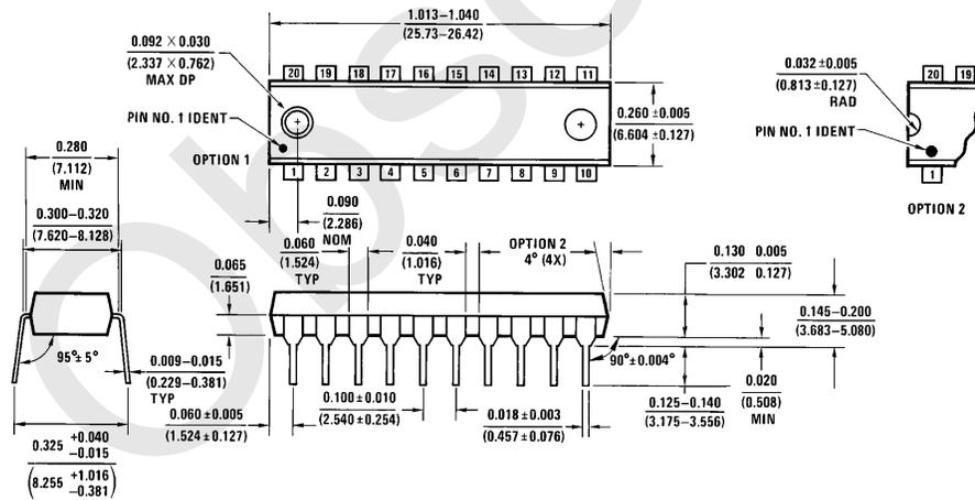
**20-Lead Molded Dual-In-Line Package (N)**
