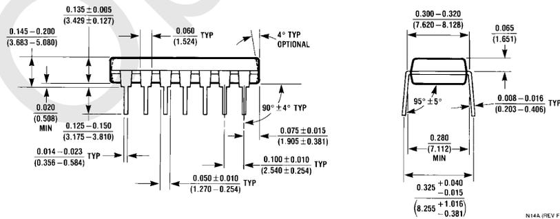
**14-Lead Molded Dual-In-Line Package (N)**
