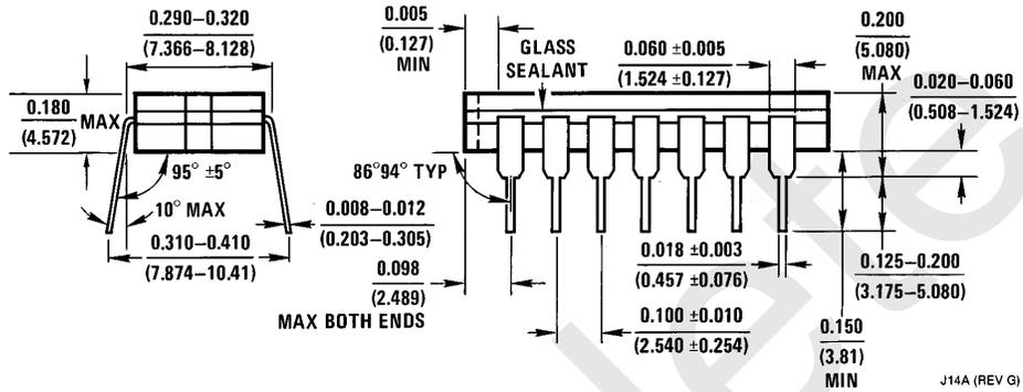
**14-Lead Ceramic Dual-In-Line Package (J)**
