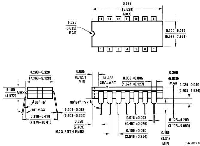
**14-Lead Ceramic Dual-In-Line Package (J)**
