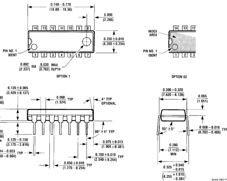
**14-Lead Molded Dual-In-Line Package (N)**
