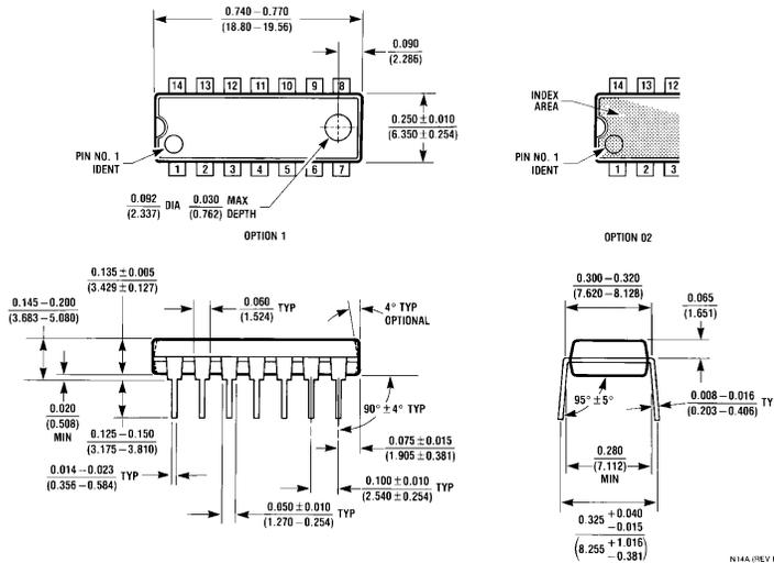
**14-Lead Molded Dual-In-Line Package (N)**
