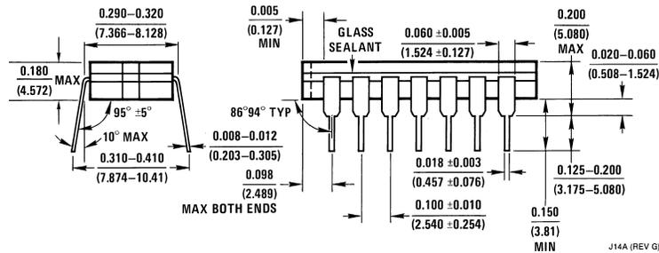
**14-Lead Ceramic Dual-In-Line Package (J)**
