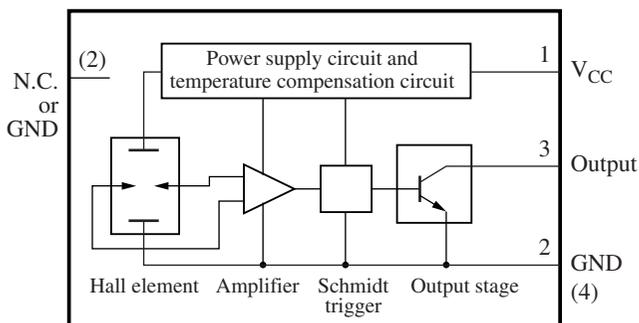
Note) The number in ( ) shows the pin number for the DN6848S.
