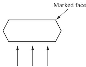
Applying direction of magnetic flux
