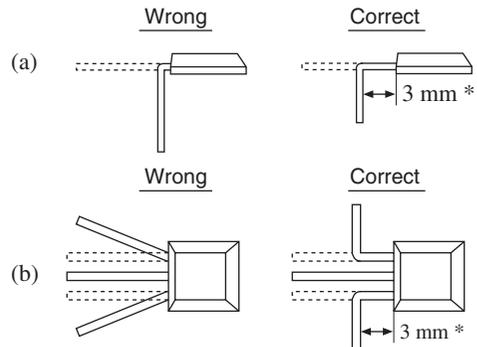
\*: The distance can be within 3 mm, if no stress is applied to the resin mold by tightly fixing the lead wires with a metallic mold or the like.
