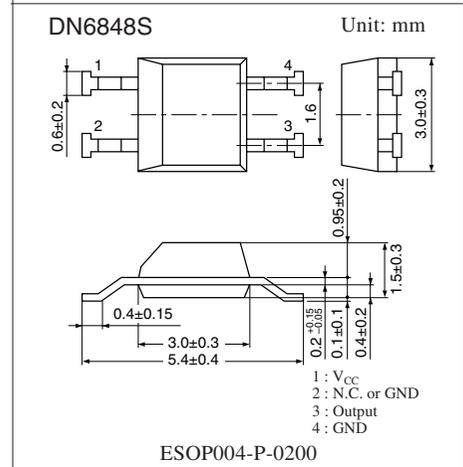
Note) The packages (SSIP003-P-0000A, SSIP003-P-0000C and ESOP004-P-0200) of this product will be changed to lead-free type (SSIP003-P-0000H, SSIP003-P-0000J and ESOP004-P-0200A). See the new package dimensions section later of this datasheet.
