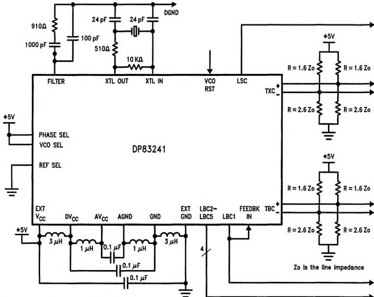
The Filter components are based on a 12.5 MHz Crystal and a 250 MHz VCO.
