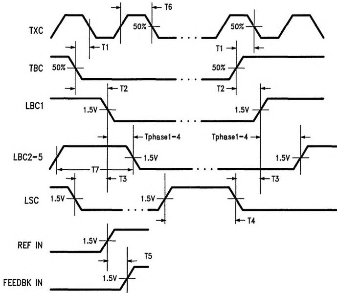
FIGURE 4-1. AC Timing Waveforms
