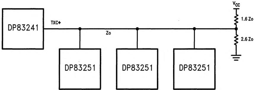
FIGURE 5-8. Proper Bus Line Termination and Connections
