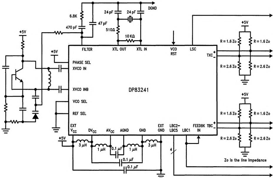
The Filter components are based on a 12.5 MHz Crystal and an external 250 MHz VCO with a gain of 40 MRad/V.
