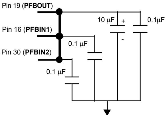
Figure 13. Power Feedback Connection
