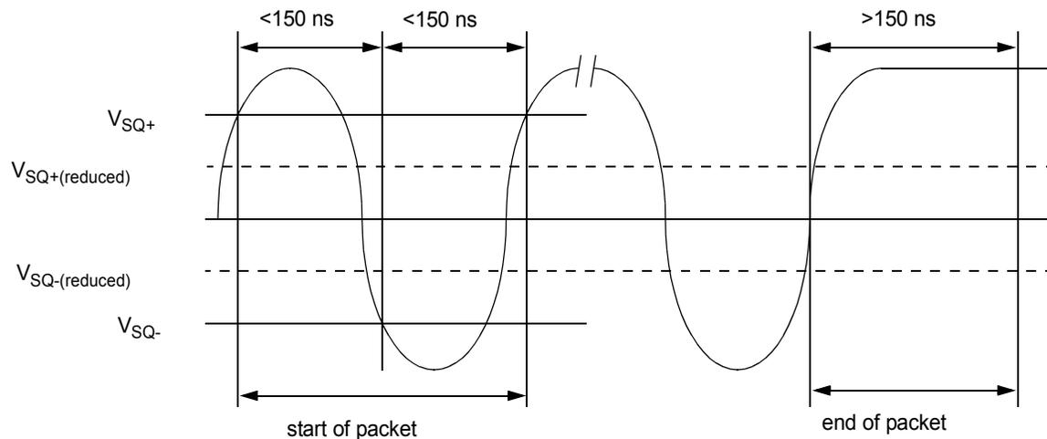
Figure 10. 10BASE-T Twisted Pair Smart Squelch Operation
