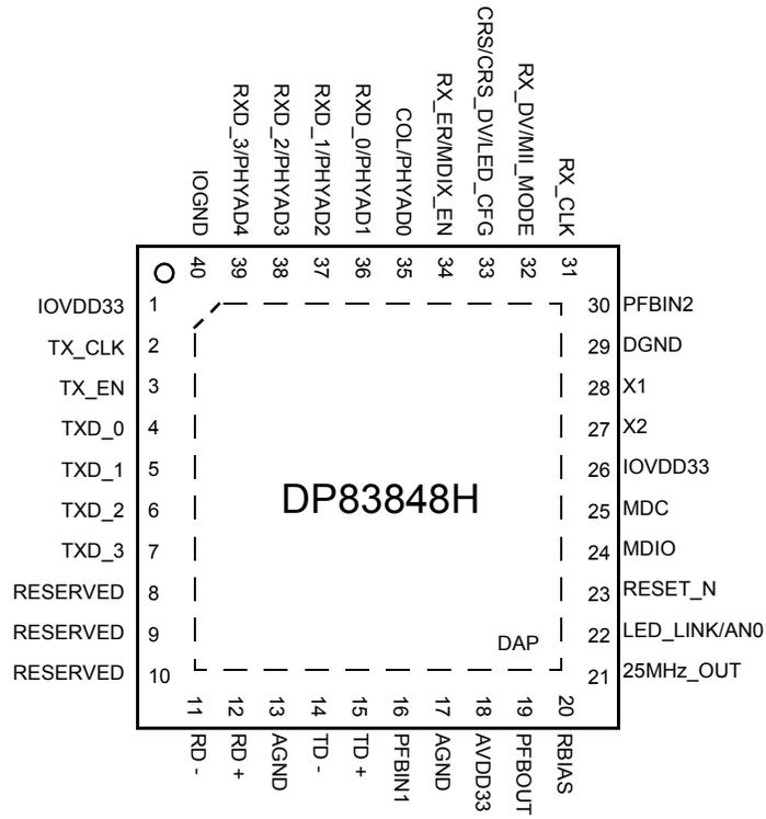
Note: Die Attached Pad (DAP) provides thermal dissipation, connection to GND plane recommended.
