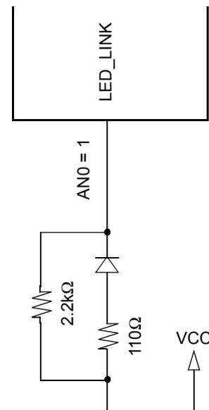
**Figure 3. AN0 Strapping and LED Loading Example**
