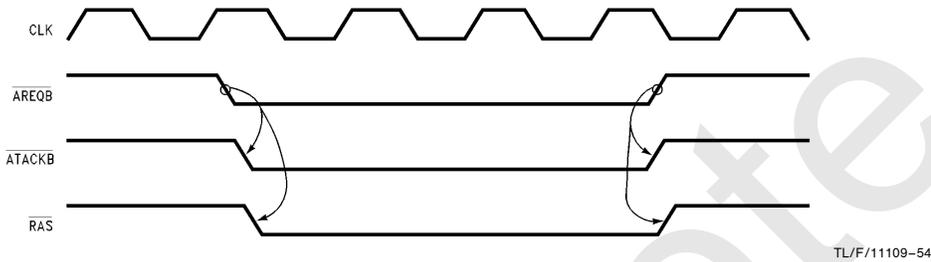
FIGURE 33a. Non-Delayed Port B Access
