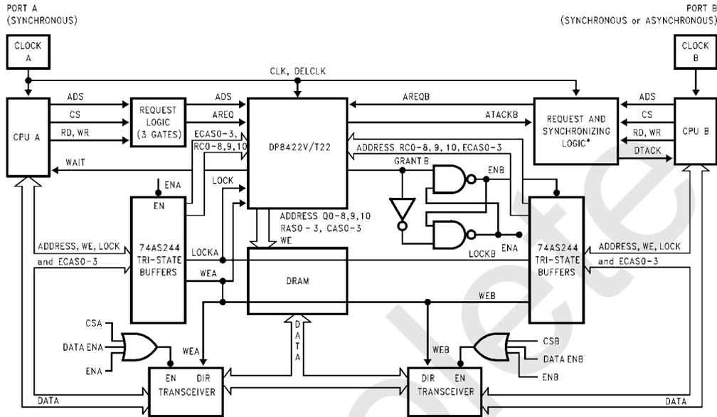
\*If Port B is synchronous the Request Synchronizing logic will not be required.
