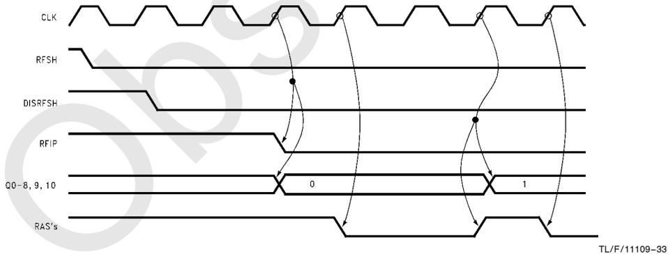
FIGURE 20b. Clearing the Refresh Counter during Burst
