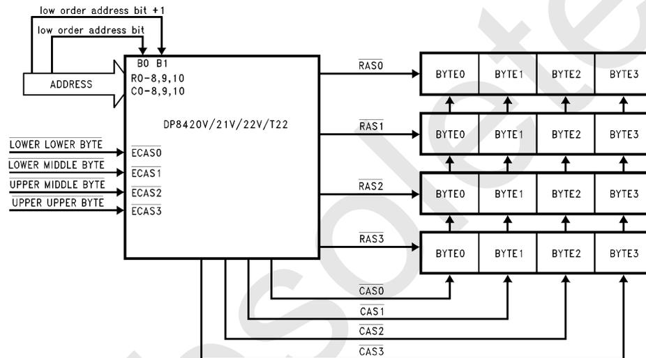
FIGURE 27. Memory Interleaving (C6, C5, C4 = 1, 1, 0 during Programming)
