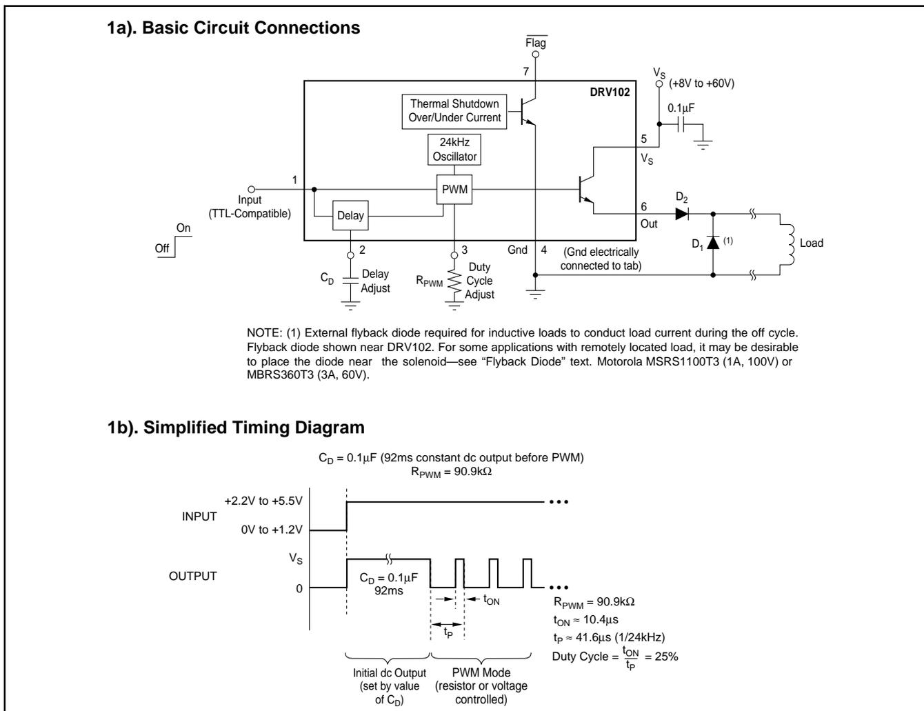
FIGURE 1. Basic Circuit Connections and Timing Diagram.
