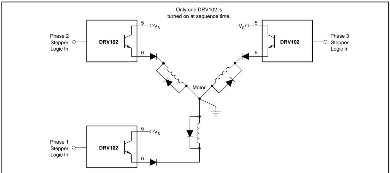
FIGURE 22. Three-Phase Stepper Motor Driver Provides High-Stepping Torque.
