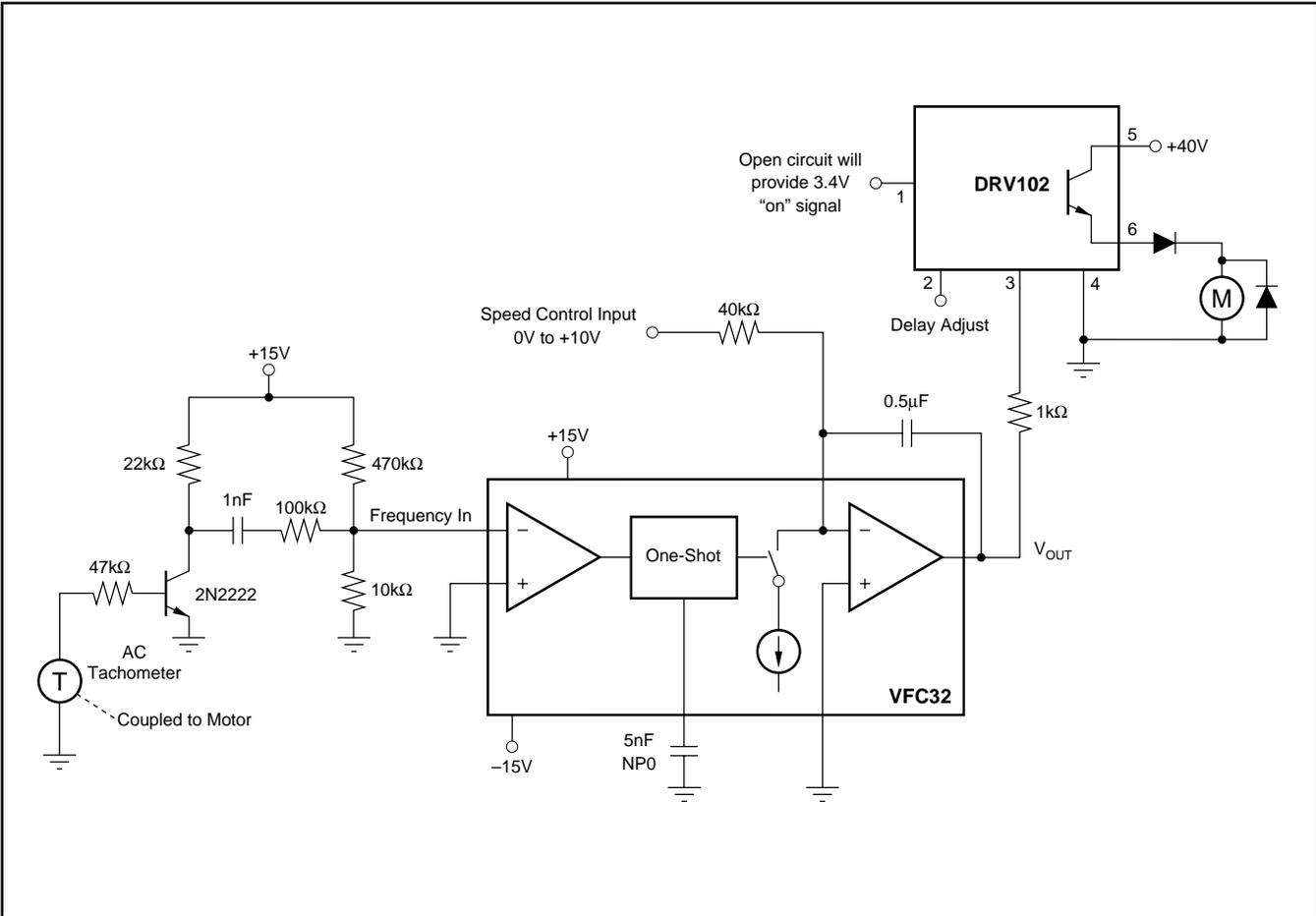
FIGURE 20. DC Motor Speed Control Using AC Tachometer.
