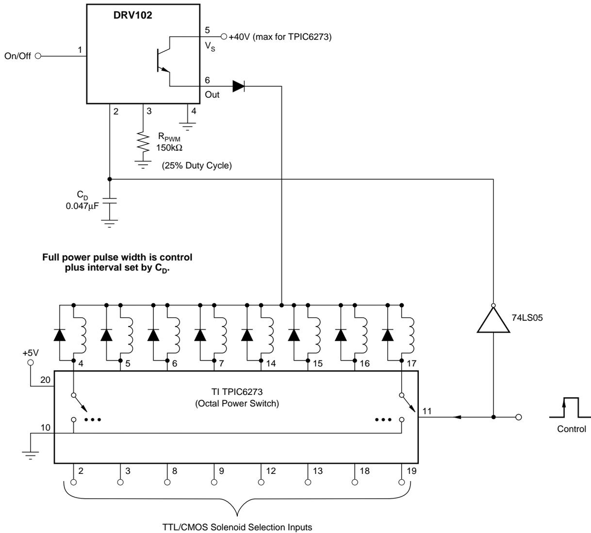
FIGURE 17. Improved Switching Time When Driving Multiple Loads.
