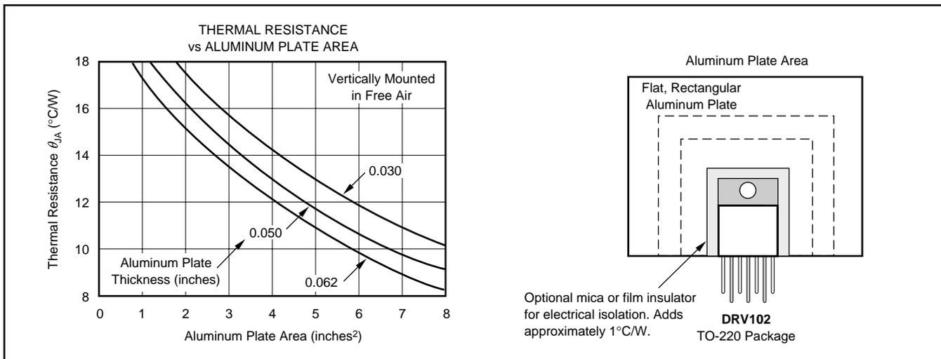
FIGURE 11. TO-220 Thermal Resistance versus Aluminum Plate Area.
