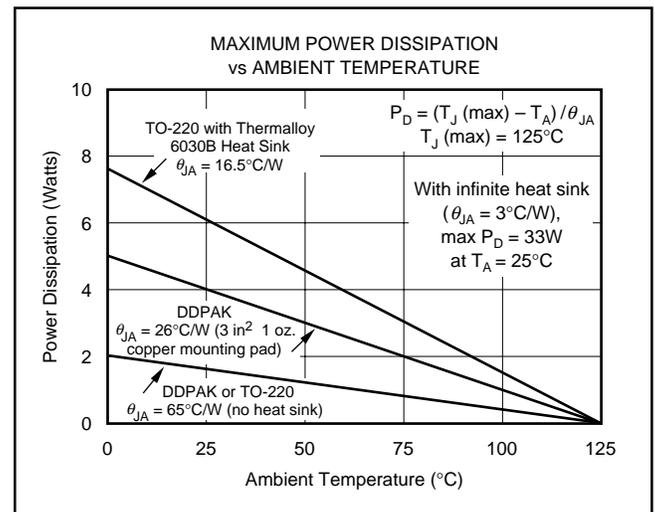
FIGURE 13. Maximum Power Dissipation versus Ambient Temperature.
