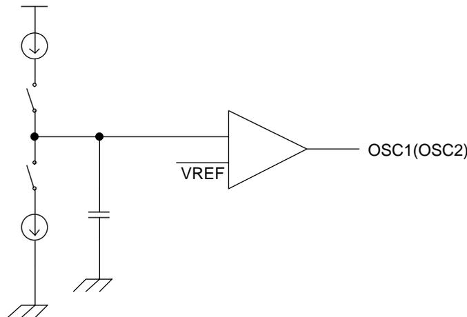
Figure 26. Oscillator Block Diagram
