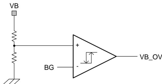
Figure 24. VB Monitor Block Diagram
