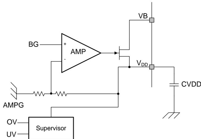
Figure 23.  $V_{DD}$  Block Diagram
