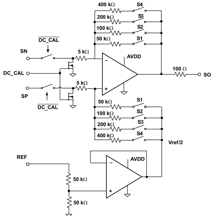
Figure 4. Current Shunt Amplifier Simplified Block Diagram
