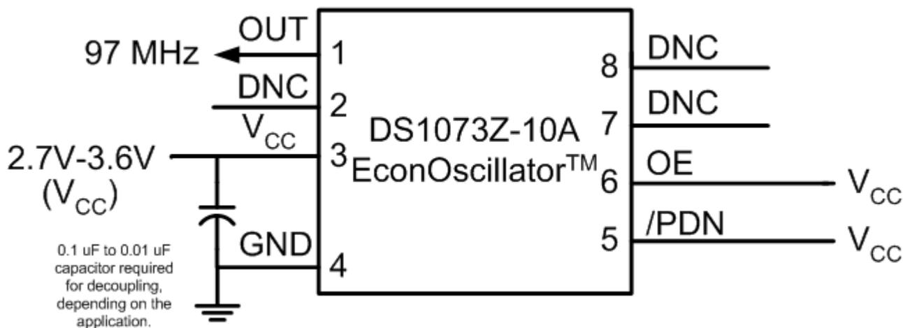
For further information on the DS1073, including AC, DC, and timing characteristics, a link to the data sheet can be found at:
