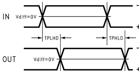
Figure 3. Propagation Delay Timing Diagram
