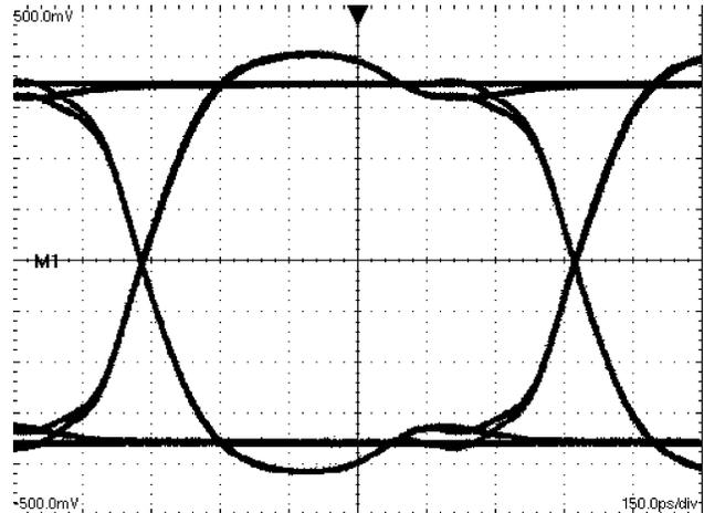
Figure 11. A 1062.5 Mbps NRZ PRBS-7 Output Eye Diagram
