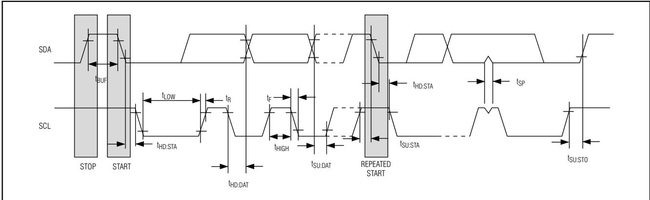
Figure 1. Data Transfer on 2-Wire Serial Bus
