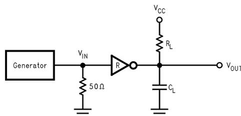
Generator characteristics for receiver input:  $f = 64\text{ kHz}$  ( $128\text{ kbits/sec}$ ),  $t_r = t_f = 200\text{ ns}$ ,  $V_{IH} = 3\text{V}$ ,  $V_{IL} = -3\text{V}$ , duty cycle = 50%.
