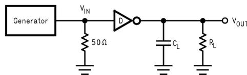
Generator characteristics for driver input:  $f = 64\text{ kHz}$  ( $128\text{ kbits/sec}$ ),  $t_r = t_f < 10\text{ ns}$ ,  $V_{IH} = 3\text{V}$ ,  $V_{IL} = 0\text{V}$ , duty cycle = 50%.
