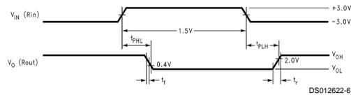
$t_r$  and  $t_f$  measured between 20% and 80% of the waveform.
