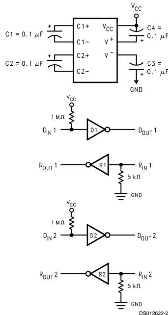
DS14C202 Low Power +5V Powered EIA/TIA-232 Dual Driver/Receiver
