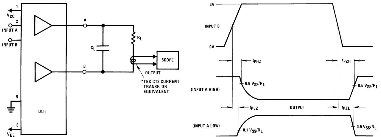
Figure 6. TRI-STATE Delays
