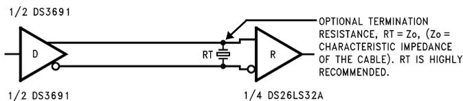
**Figure 9. RS-422 Point to Point Application**
