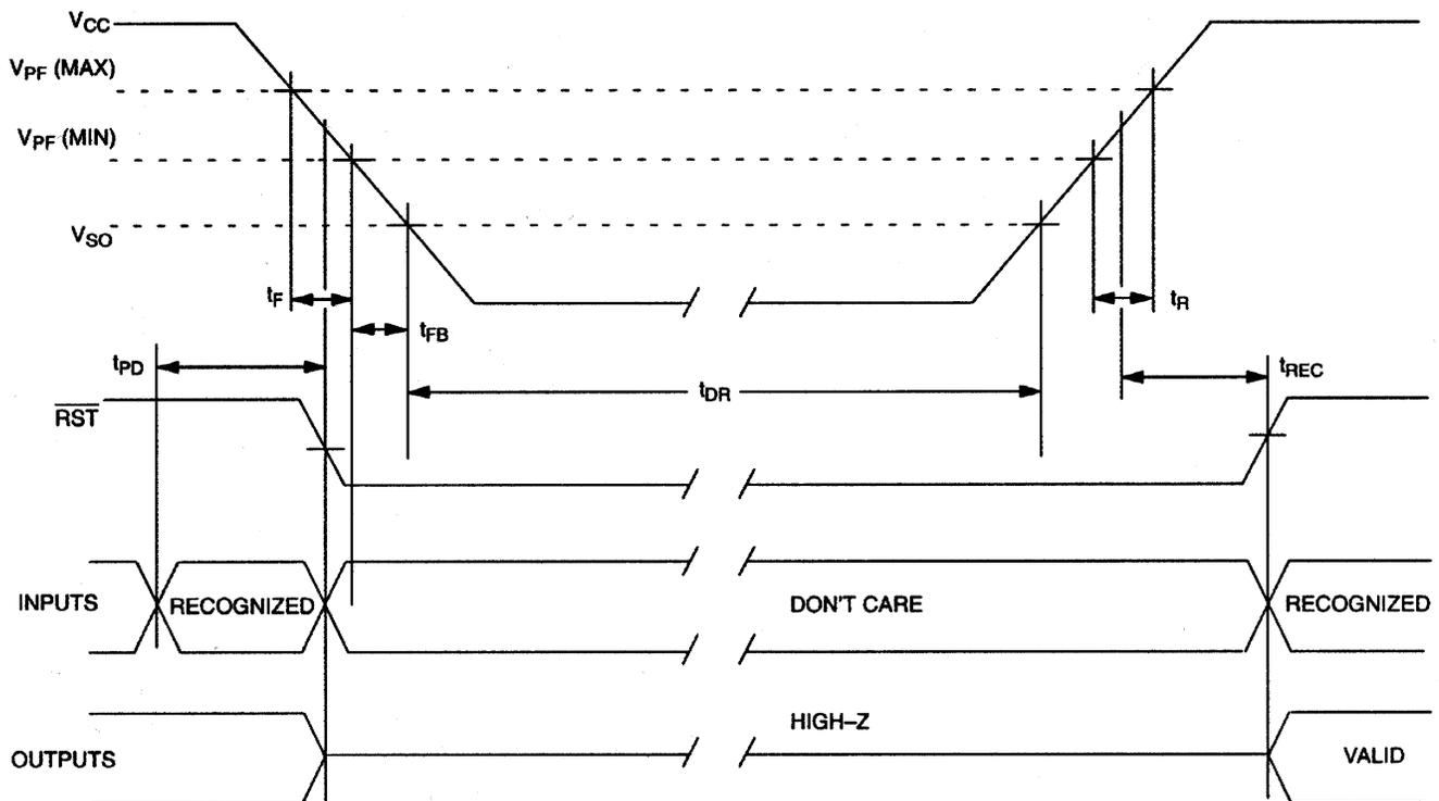
**POWER-UP/DOWN CHARACTERISTICS**(Over the Operating Range;  $V_{CC} = 3.3V \pm 10\%$ )
