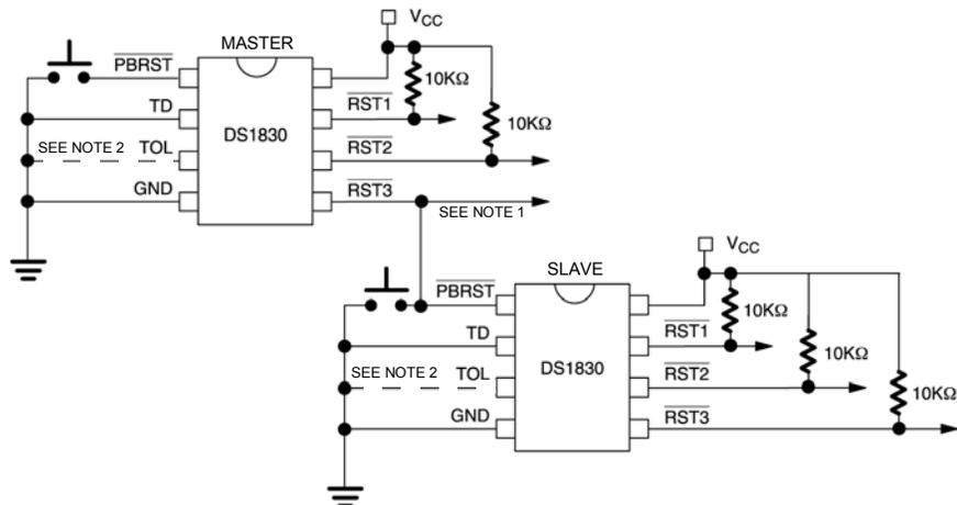
**Note 1:** The RST3 output tied to the pushbutton reset would be pulled to  $V_{CC}$  through the 40KΩ resistor in the pushbutton input. If a stronger pull-up is required an additional pull-up resistor could be added.
