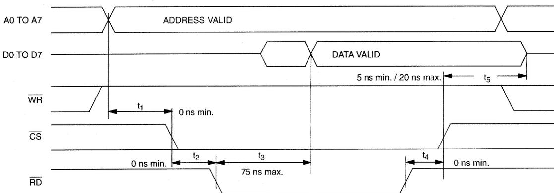
**INTEL BUS WRITE AC TIMING (BTS=0/MUX=0) Figure 14-11**
