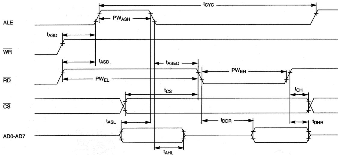
**INTEL BUS WRITE AC TIMING (BTS=0/MUX=1) Figure 14-2**
