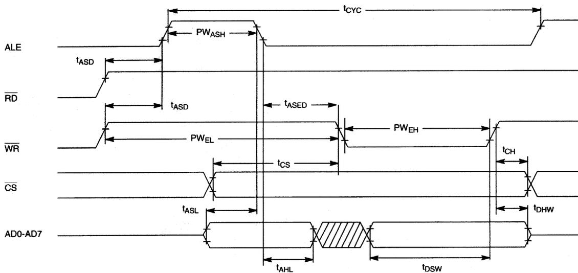
**MOTOROLA BUS AC TIMING (BTS=1/MUX=1) Figure 14-3**
