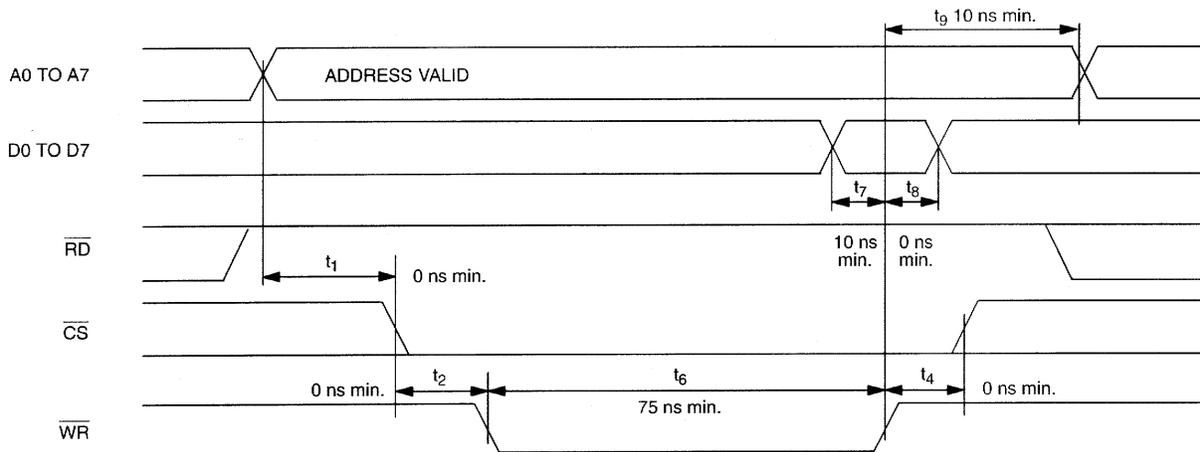
**MOTOROLA BUS READ AC TIMING (BTS=1/MUX=0) Figure 14-12**
