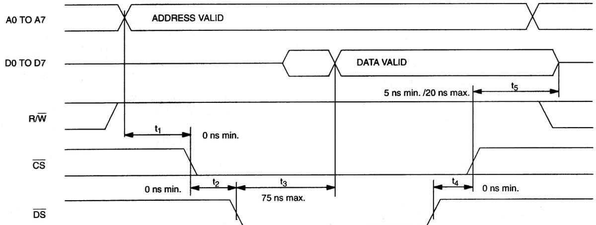
**MOTOROLA BUS WRITE AC TIMING (BTS=1/MUX=0) Figure 14-13**
