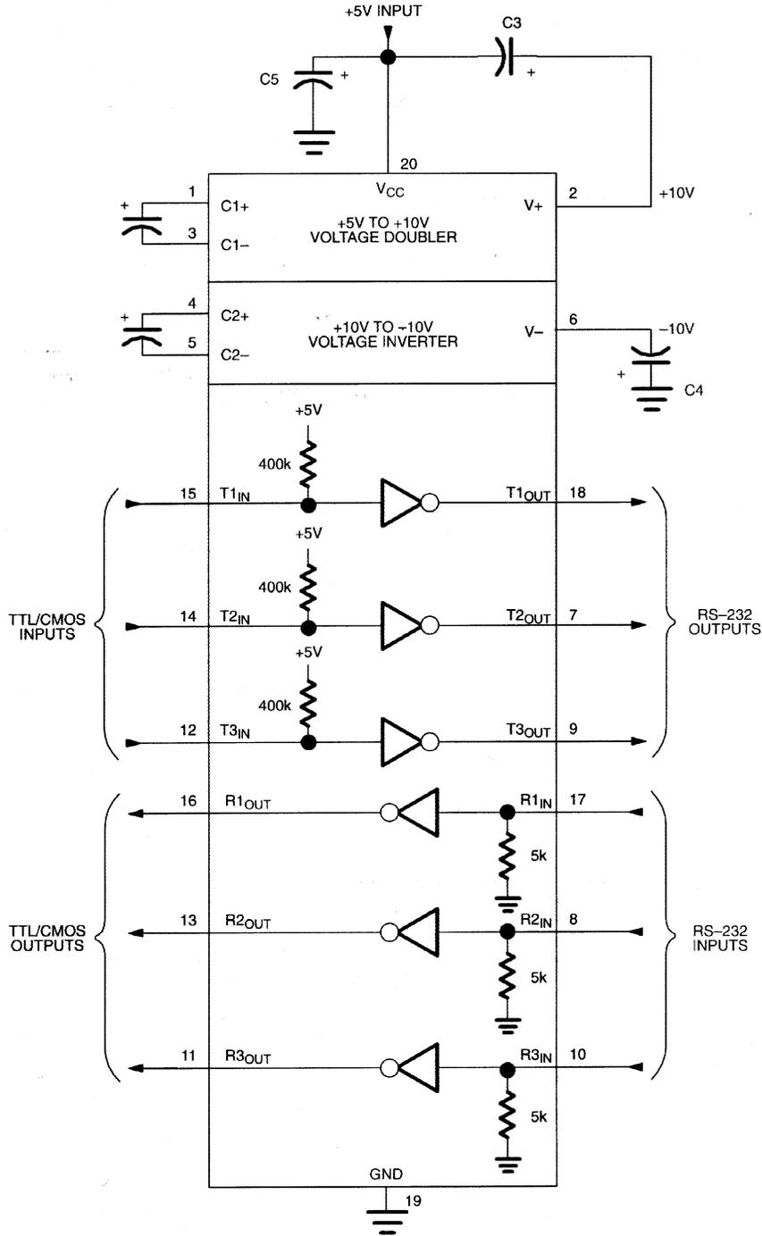
NOTE: C5 is a recommended decoupling capacitor which is the same value as C1, C2, C3, and C4.
