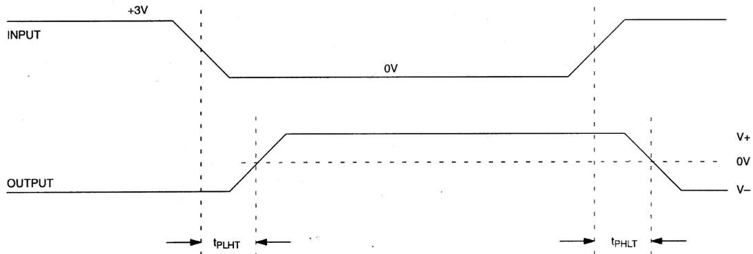
**RECEIVER PROPAGATION DELAY TIMING Figure 3**
