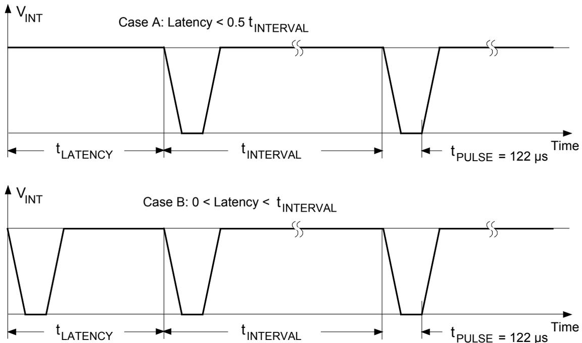
The latency depends on the selected interrupt interval (IS0 to IS2 settings) and the contents of the RTC counter at the time of writing the device control byte. In Case A, the flip-flop that determines the interval duration is reset and toggles before half of the interval time is over. In Case B, this flip-flop is set that generates an immediate interrupt pulse; the latency, therefore, can be up to one full interval duration.
