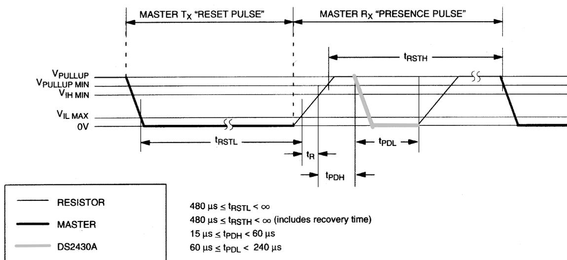
In order not to mask interrupt signaling by other devices on the 1-Wire bus,  $t_{RSTL} + t_R$  should always be less than 960  $\mu\text{s}$ .
