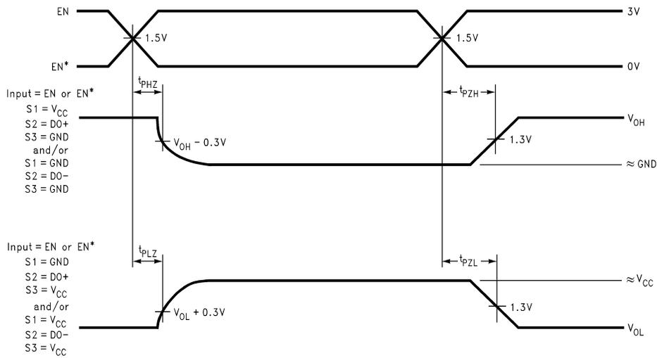
**Figure 6. Driver Single-Ended TRI-STATE Waveforms**
