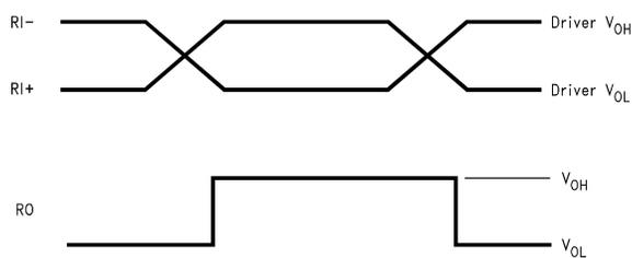
**Figure 7. Typical Receiver Output Waveforms**
