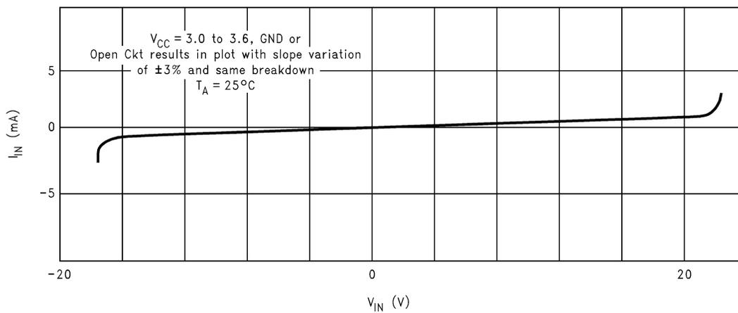
Figure 10. Receiver I<sub>IN</sub> vs V<sub>IN</sub> (Power On or Power Off)
