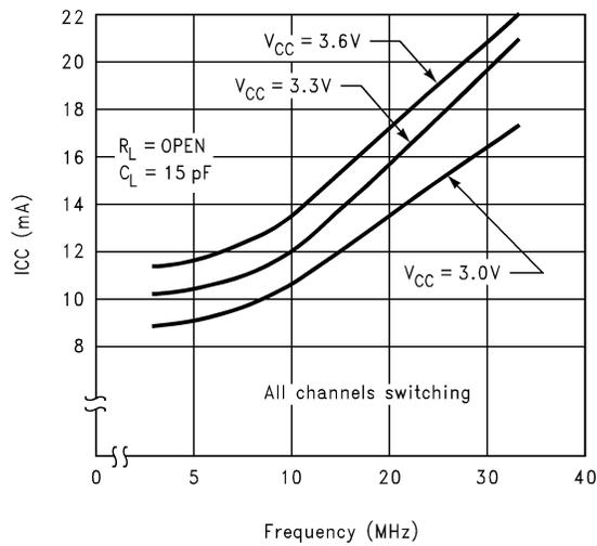
Figure 9. Typical I<sub>CC</sub> vs Frequency
