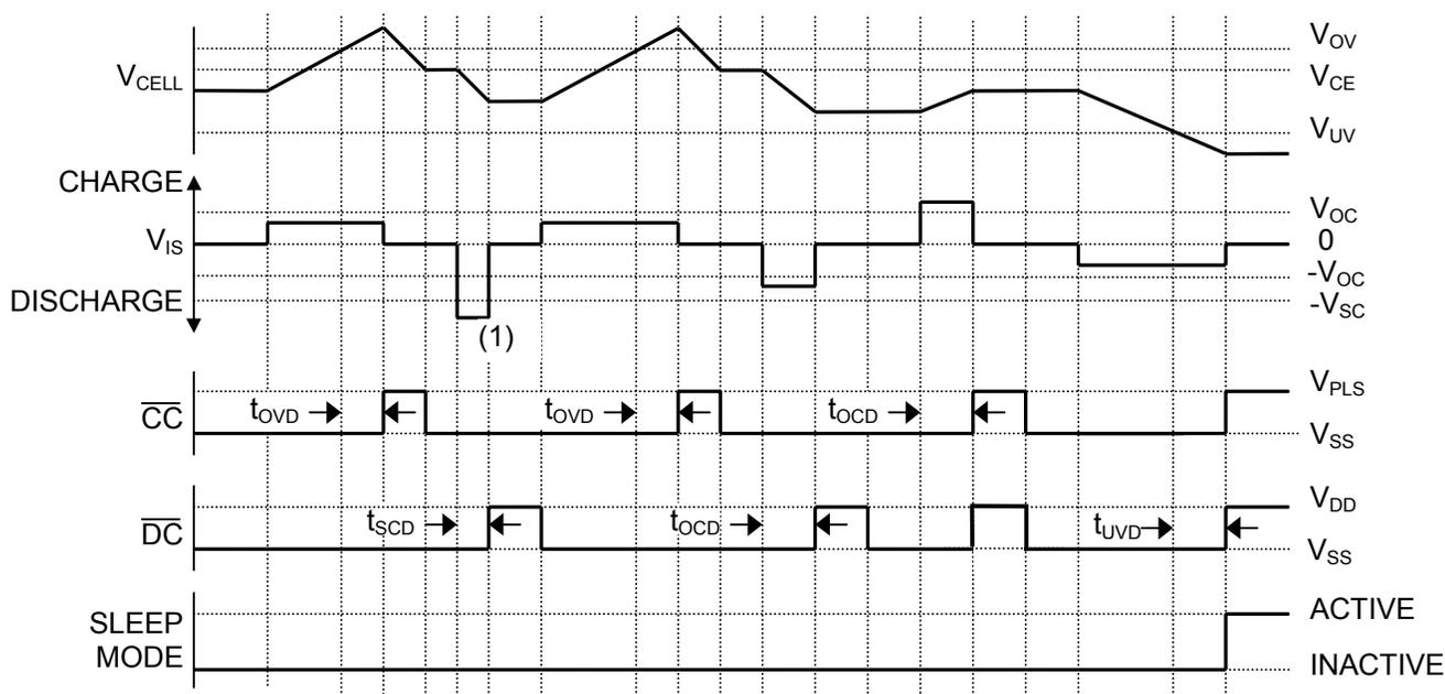
(1) To allow the device to react quickly to short circuits, detection occurs on the SNS pin rather than on the filtered IS1 and IS2 pins. The actual short-circuit detect condition is  $V_{SNS} > V_{SC}$ .
