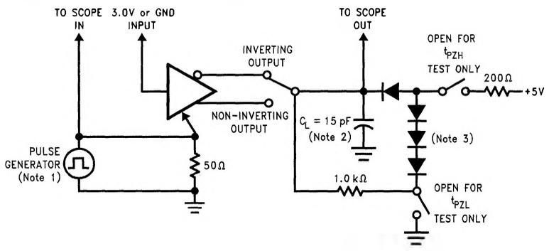
**FIGURE 2. TRI-STATE Enable Test Circuit and Waveforms**
