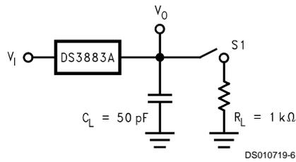
FIGURE 4. Receiver Propagation Delay Set-Up
