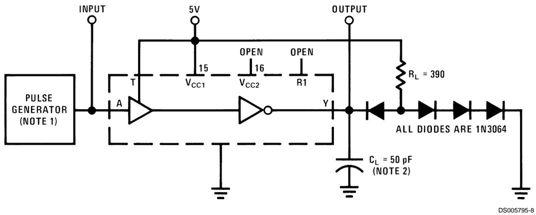
**Note 1:** The pulse generator has the following characteristics:  $Z_{OUT} = 50\Omega$ ,  $t_W = 200$  ns, duty cycle  $\leq 20\%$ .
