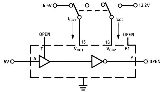
All four line receivers are tested simultaneously.
