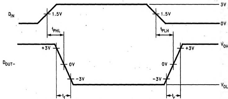
FIGURE 3. Driver Propagation Delay and Transition Time Waveform
