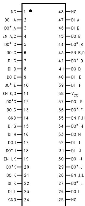
**Figure 1. 48-Pin SSOP Package
