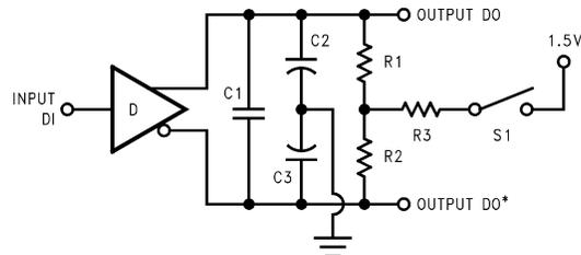
C1 = C2 = C3 = 40 pF (including Probe and Jig Capacitance), R1 = R2 = 50Ω, R3 = 500Ω
