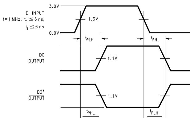
Figure 4. Propagation Delays
