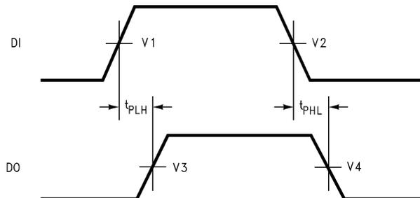
**Figure 10. Waveforms for Circuit 1 – Propagation Delay Waveforms for Circuit 1 and Circuit 2**
