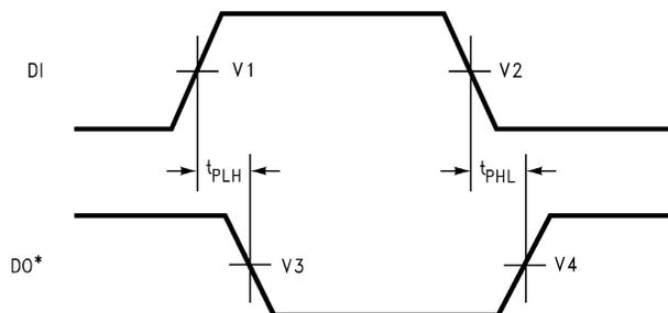
**Figure 11. Waveforms for Circuit 2 – Propagation Delay Waveforms for Circuit 1 and Circuit 2**
