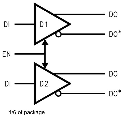
**Figure 2. Functional Diagram**
