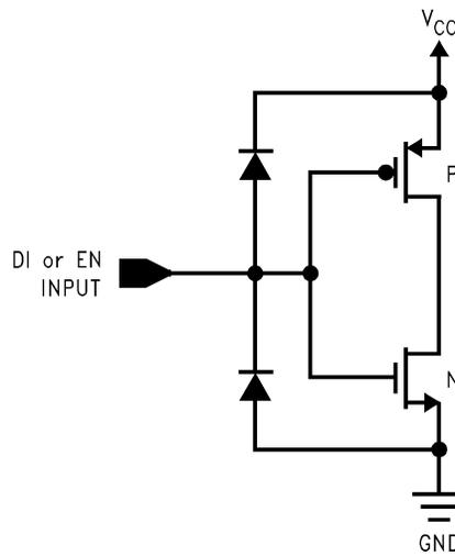
Figure 17. Driver Input or Driver Enable Equivalent Circuit
