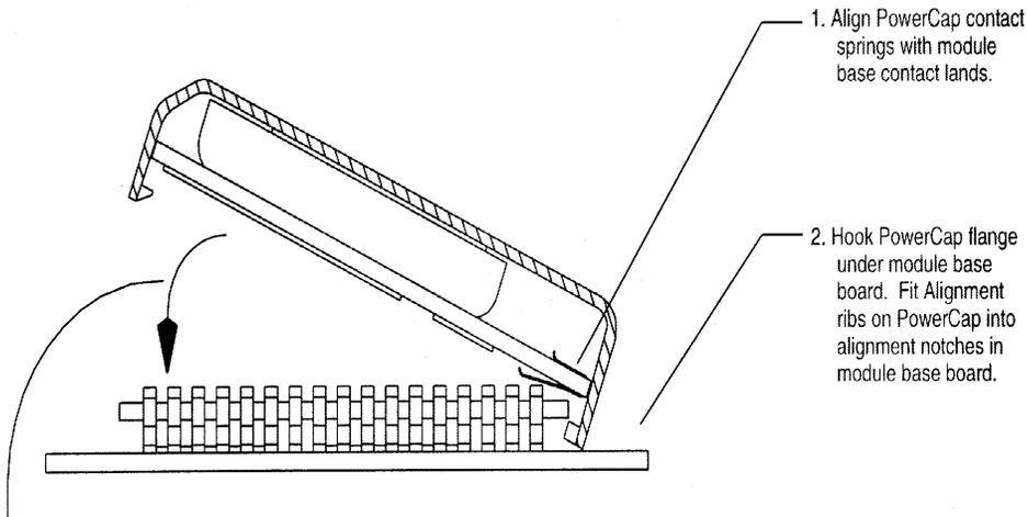
3. Pushdown and forward with screwdriver while inserting the PowerCap. This action will "open" the attachment feature.
