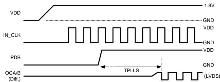
Figure 8. Start Up / Phase Lock Loop Set Time
