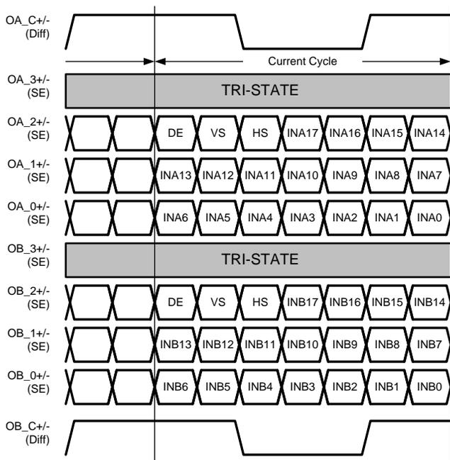
Figure 16. Dual Pixel / 18bpp LVDS Mapping
