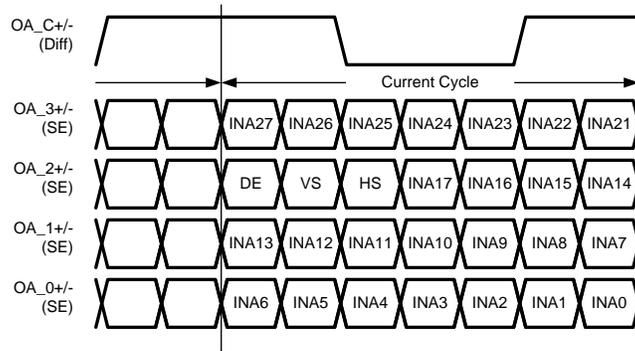
Figure 17. Single Pixel / 24bpp LVDS Mapping
