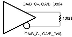
Figure 4. DS90C187 (Transmitter) LVDS Output Load
