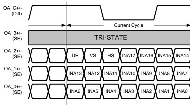
Figure 18. Single Pixel / 18bpp LVDS Mapping
