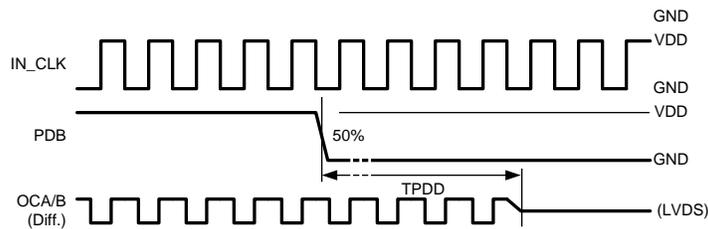
Figure 9. Sleep Mode / Power Down Delay
