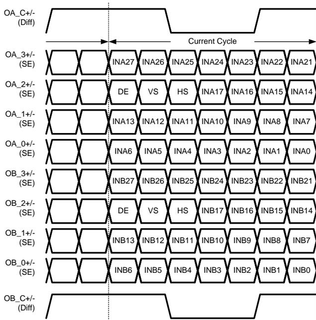
Figure 15. Dual Pixel / 24bpp LVDS Mapping
