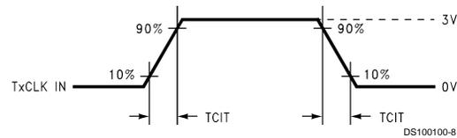
FIGURE 5. DS90C383A/DS90CF383A (Transmitter) Input Clock Transition Time
