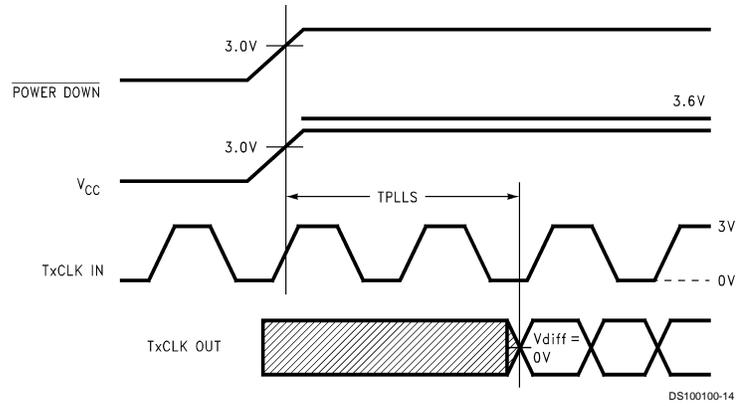
**FIGURE 8. DS90C383A/DS90CF383A (Transmitter) Phase Lock Loop Set Time**
