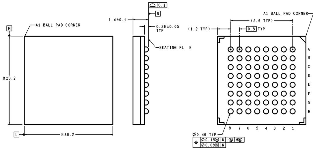
DIMENSIONS ARE IN MILLIMETERS
