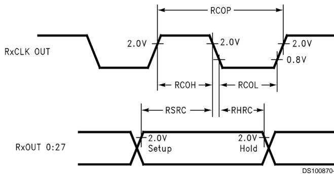
**FIGURE 5. DS90CF384A/DS90CF364A (Receiver) Setup/Hold and High/Low Times**
