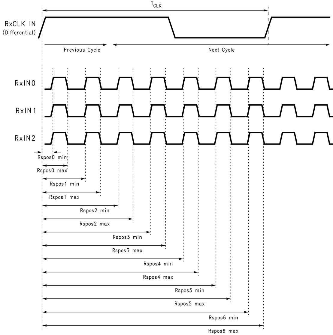
FIGURE 12. DS90CF364A (Receiver) LVDS Input Strobe Position
