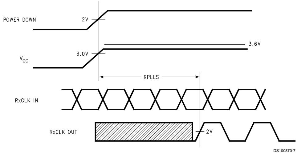
FIGURE 7. DS90CF384A/DS90CF364A (Receiver) Phase Lock Loop Set Time
