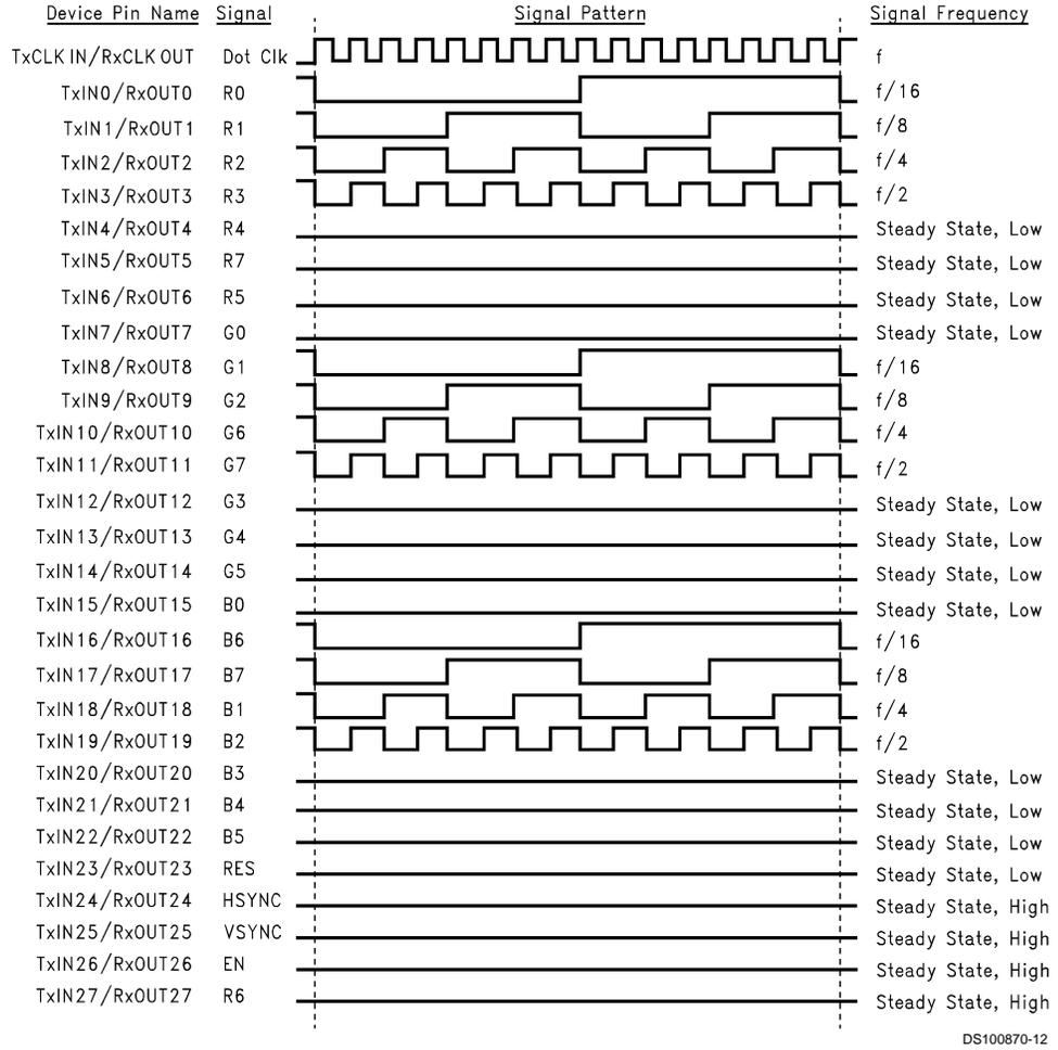
FIGURE 2. "16 Grayscale" Test Pattern (DS90CF384A)(Notes 5, 6, 7, 8)
