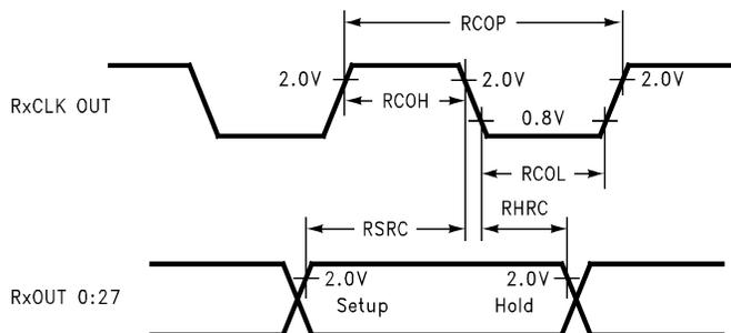
Figure 13. DS90CF562 (Receiver) Setup/Hold and High/Low Times
