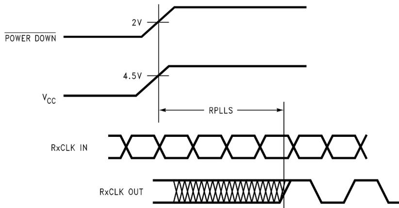
Figure 17. DS90CF562 (Receiver) Phase Lock Loop Set Time
