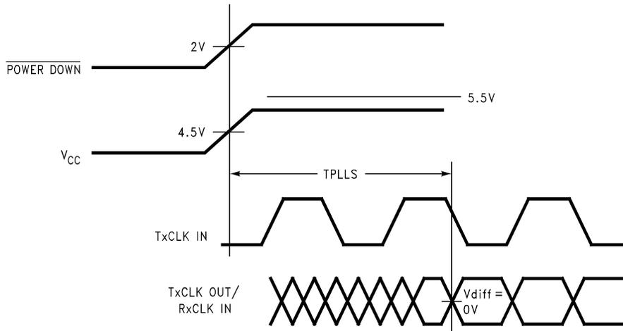
Figure 16. DS90CF561 (Transmitter) Phase Lock Loop Set Time
