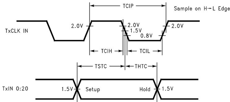
Figure 12. DS90CF561 (Transmitter) Setup/Hold and High/Low Times
