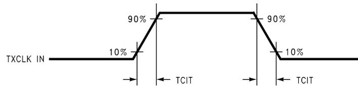
Figure 10. DS90CF561 (Transmitter) Input Clock Transition Time
