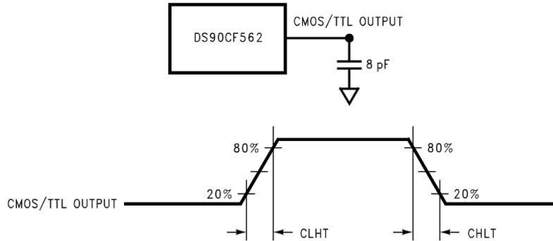
Figure 9. DS90CF562 (Receiver) CMOS/TTL Output Load and Transition Timing
