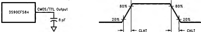
FIGURE 4. DS90CF584 (Receiver) CMOS/TTL Output Load and Transition Times
