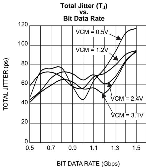
Total Jitter measured at 0V differential while running a PRBS 2<sup>23</sup>-1 pattern in single channel repeater mode. V<sub>CC</sub> = 3.3V, T<sub>A</sub> = +25°C, V<sub>ID</sub> = 0.5V
