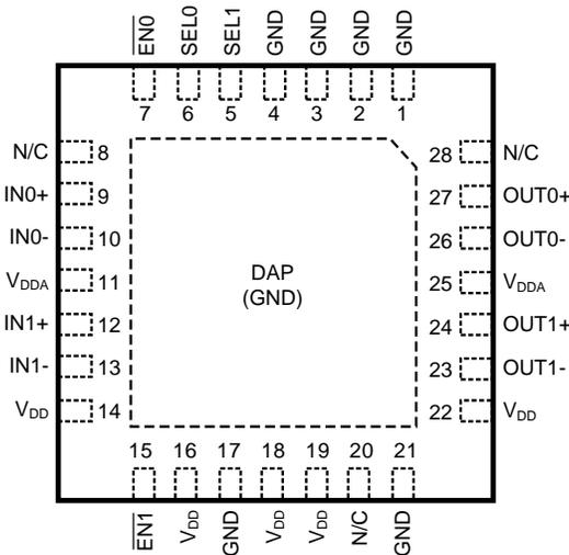
**Figure 2. UQFN Top View
