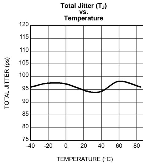
Total Jitter measured at 0V differential while running a PRBS 2<sup>23</sup>-1 pattern in dual channel repeater mode. V<sub>CC</sub> = 3.3V, V<sub>ID</sub> = 0.5V, V<sub>CM</sub> = 1.2V, 1.5 Gbps data rate
