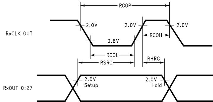
Figure 11. DS90CR286 (Receiver) Setup/Hold and High/Low Times
