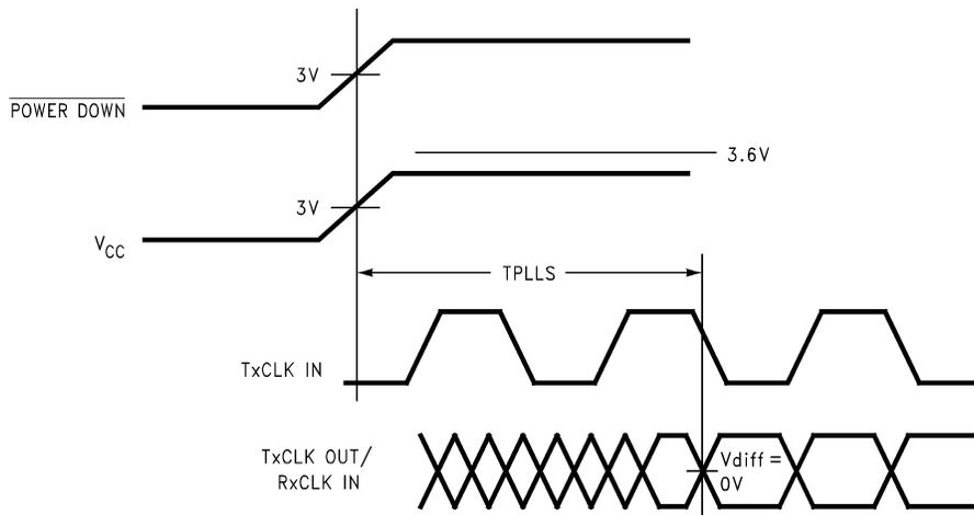
Figure 14. DS90CR285 (Transmitter) Phase Lock Loop Set Time
