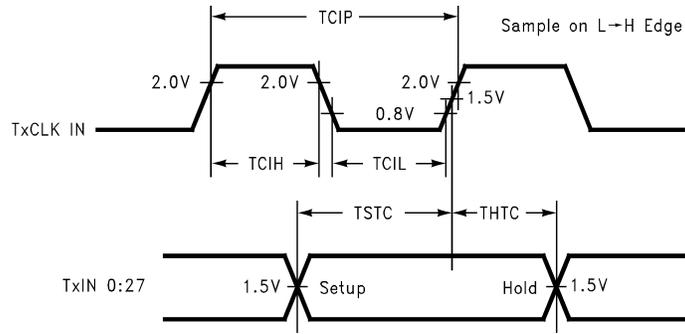
Figure 10. DS90CR285 (Transmitter) Setup/Hold and High/Low Times
