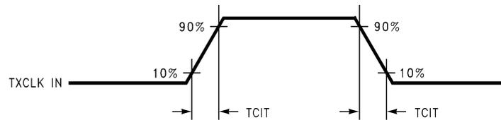
Figure 8. DS90CR285 (Transmitter) Input Clock Transition Time
