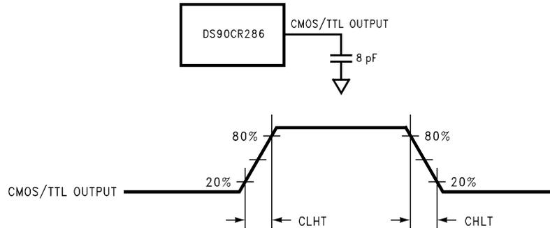
Figure 7. DS90CR286 (Receiver) CMOS/TTL Output Load and Transition Times
