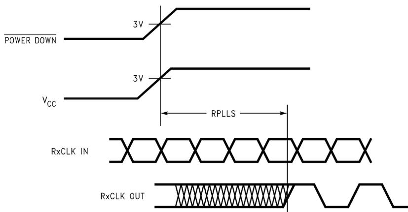
Figure 15. DS90CR286 (Receiver) Phase Lock Loop Set Time
