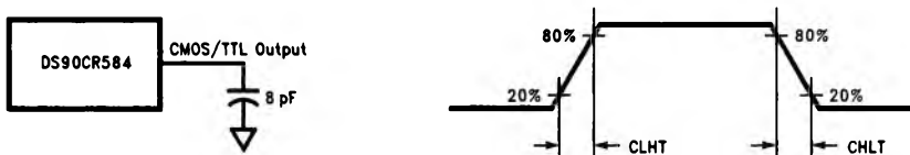
FIGURE 4. DS90CR584 (Receiver) CMOS/TTL Output Load and Transition Times
