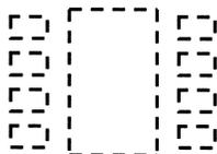
**Figure 6. WSON Thermal Land Pad and Pin Pads**
