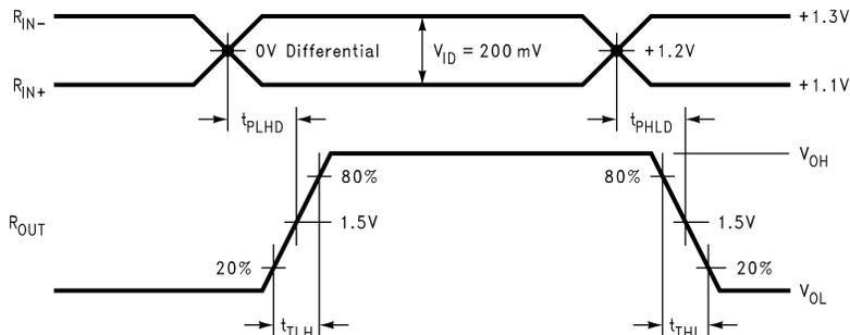
**Figure 4. Receiver Propagation Delay and Transition Time Waveforms**
