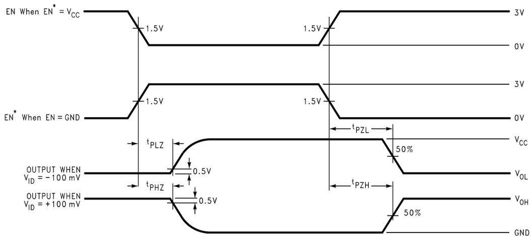
Figure 4. Receiver TRI-STATE Delay Waveforms
