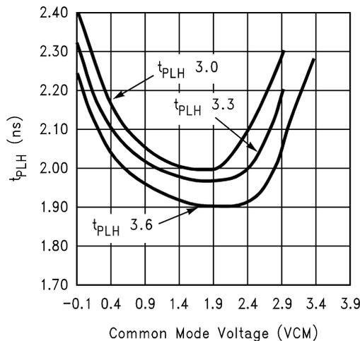
Figure 9. Variation in Low to High Propagation Delay versus  $V_{CM}$
