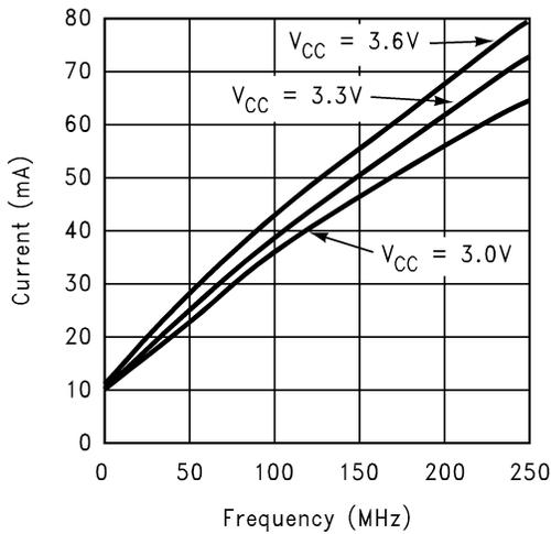
Figure 5.  $I_{CC}$  vs Frequency, four channels switching
