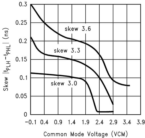
Figure 7. Typical Pulse Skew variation versus common-mode voltage
