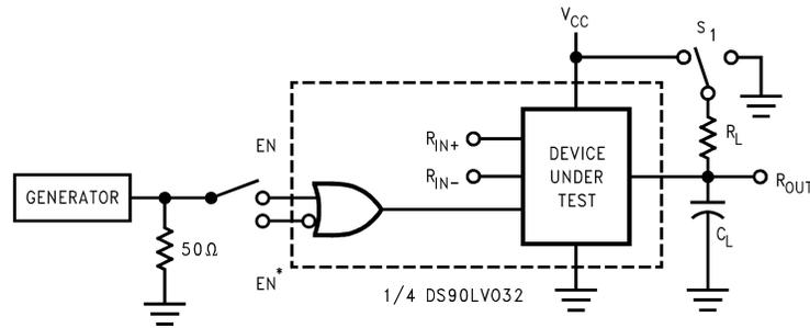
$C_L$  includes load and test jig capacitance.
