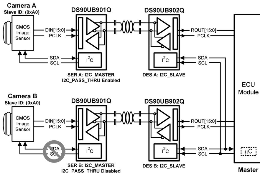
Figure 31. I<sup>2</sup>C Pass Through
