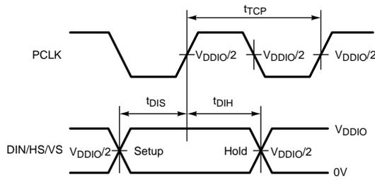
Figure 12. Serializer Setup/Hold Times
