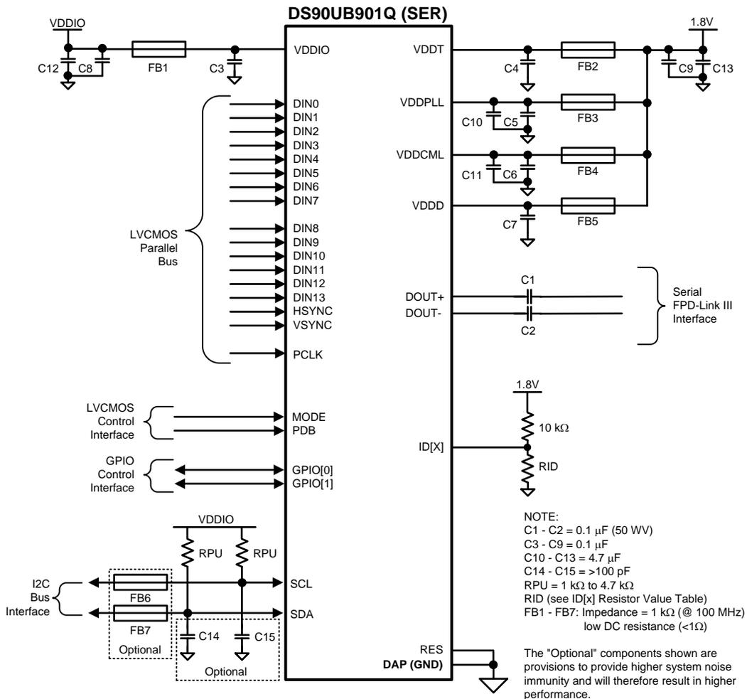
Figure 39. DS90UB901Q Typical Connection Diagram — Pin Control
