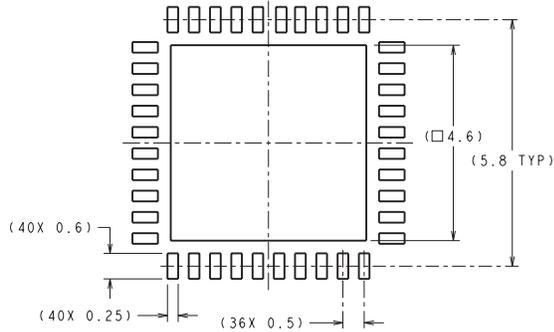
DIMENSIONS ARE IN MILLIMETERS
