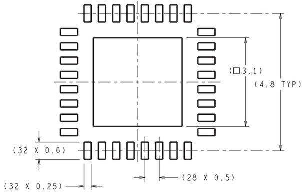
DIMENSIONS ARE IN MILLIMETERS
