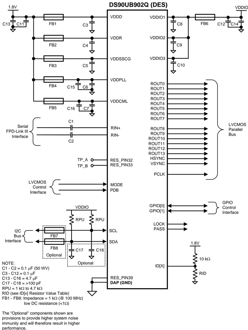
Figure 40. DS90UB902Q Typical Connection Diagram — Pin Control
