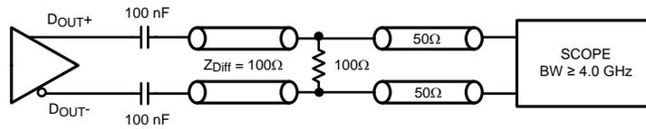
Figure 7. Serializer CML Output Load and Transition Times
