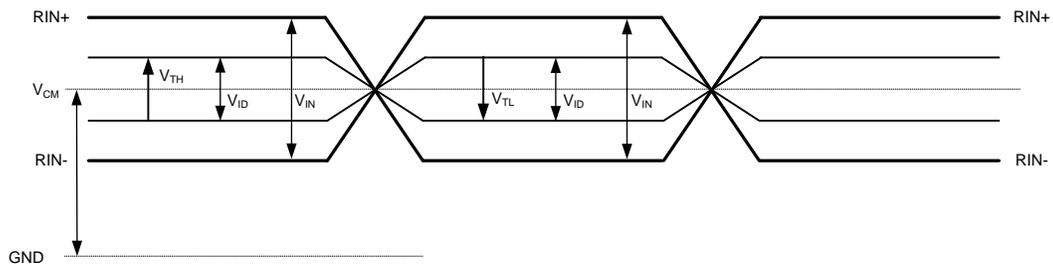
Figure 10. Differential VTH/VTL Definition Diagram
