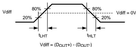
Figure 6. Serializer CML Output Load and Transition Times
