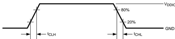
Figure 4. LVCMOS Transition Times
