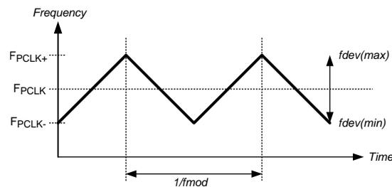
Figure 13. SSCG Waveform
