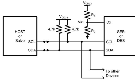
**Figure 20. Serial Control Bus Connection**
