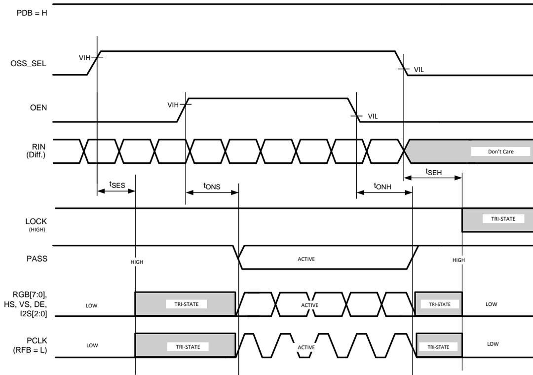
Figure 8. Output State (Setup and Hold) Times
