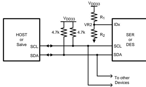
Figure 20. Serial Control Bus Connection
