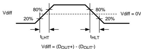
Figure 8. Serializer CML Output Load and Transition Times
