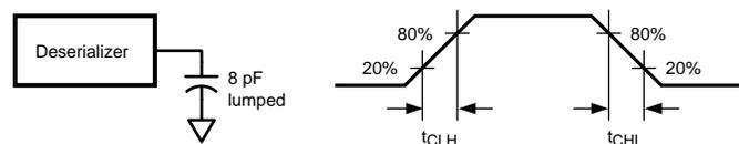
Figure 18. Deserializer LVC MOS Output Load and Transition Times
