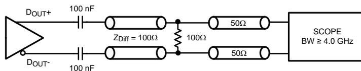
Figure 9. Serializer CML Output Load and Transition Times
