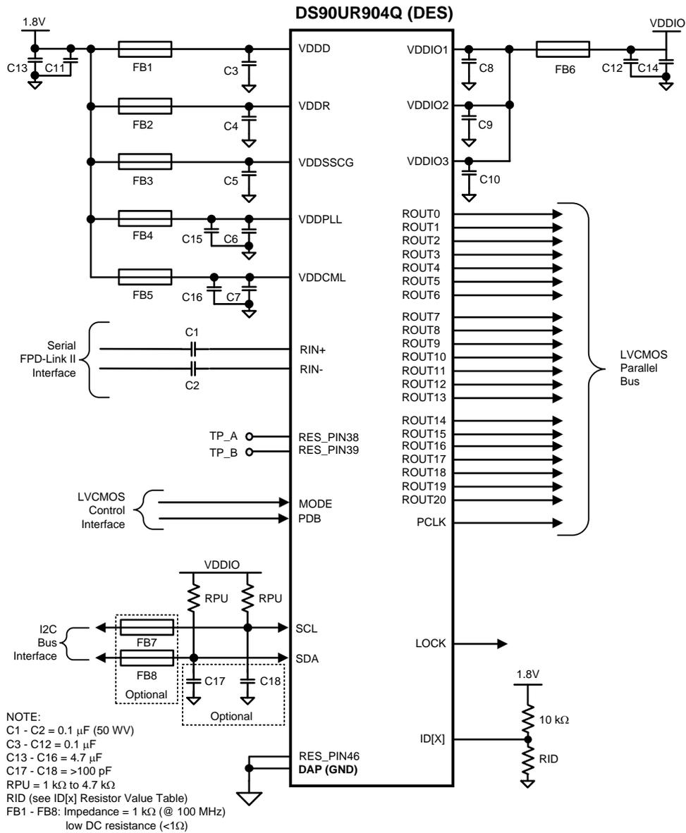
**Figure 32. DS90UR904Q Typical Connection Diagram — Pin Control 48-Pin WQFN (RHS Package)**
