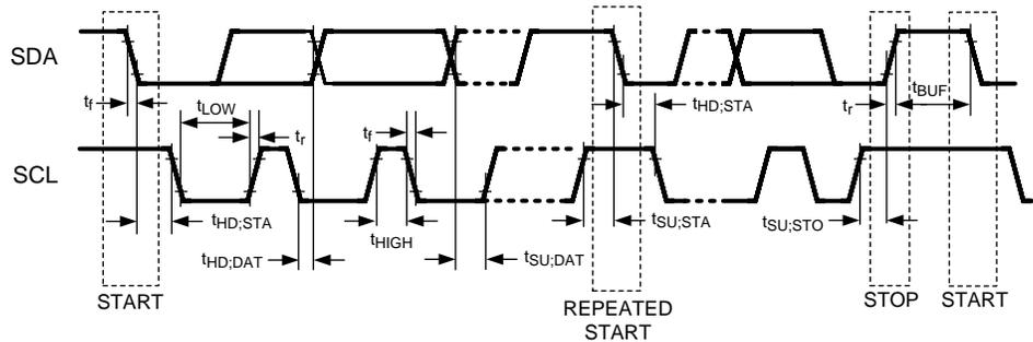
**Figure 6. Serial Control Bus Timing**
