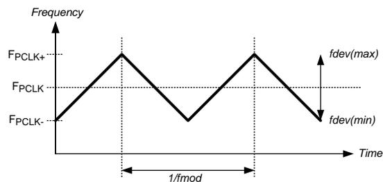
**Figure 17. SSCG Waveform**
