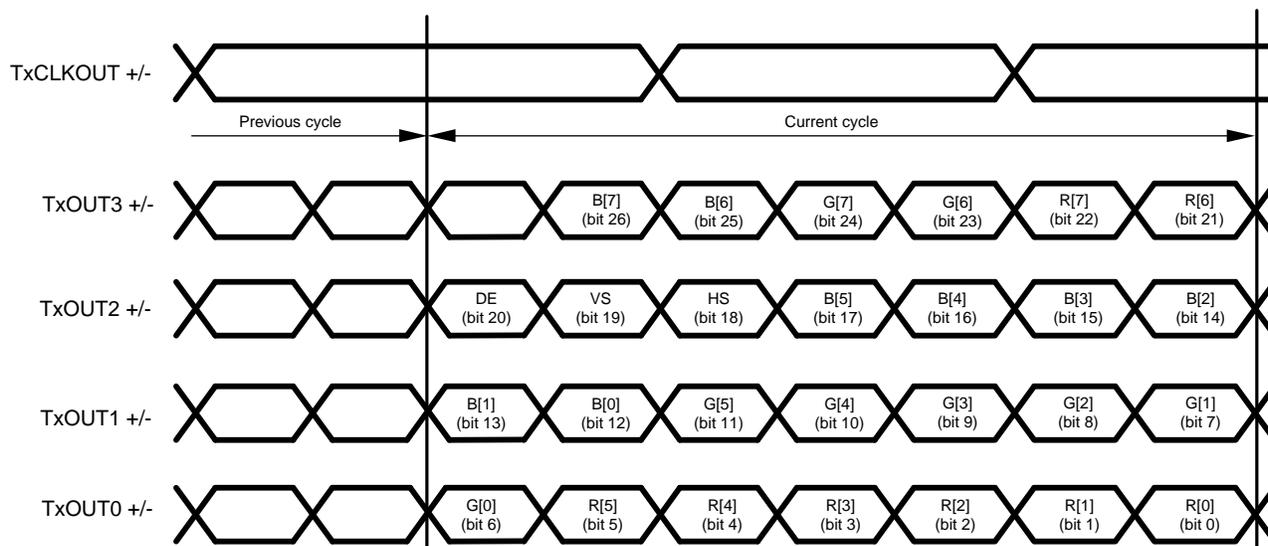
**Figure 16. 8-bit FPD-Link Mapping: MSB's on TxOUT3**
