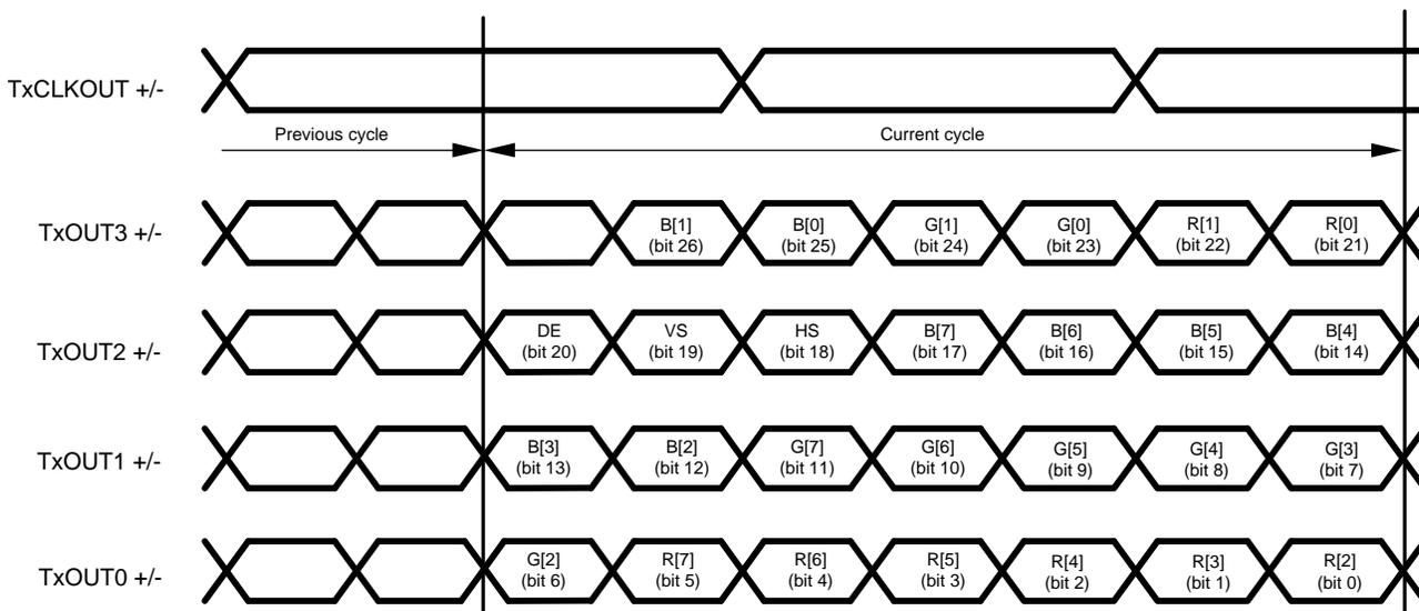
Figure 15. 8-bit FPD-Link Mapping: LSB's on TxOUT3
