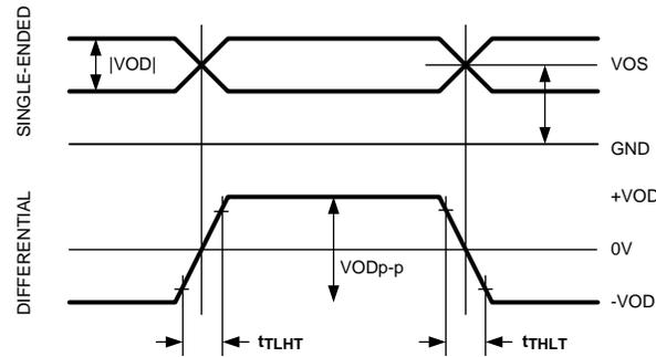
Figure 8. FPD-Link (LVDS) Single-ended and Differential Waveforms
