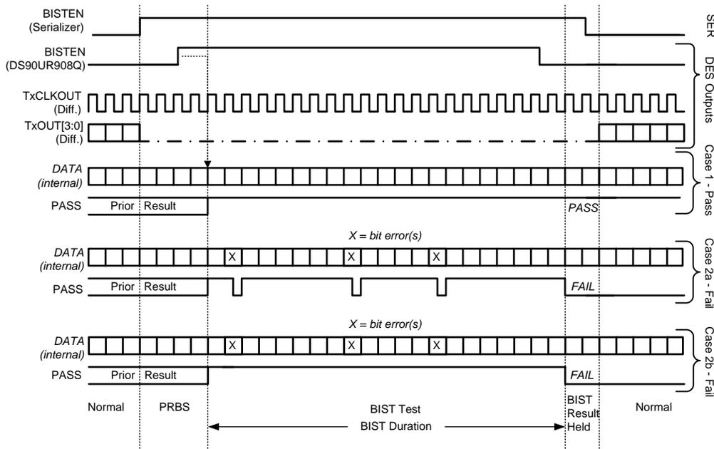
Figure 20. BIST Waveforms
